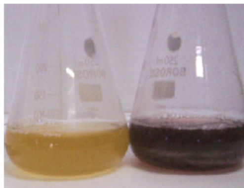
Silver nitrate (1 mmol l -1 ) in conical flasks before (left) and after (right) exposure to Phoma glomerata culture supernatant
